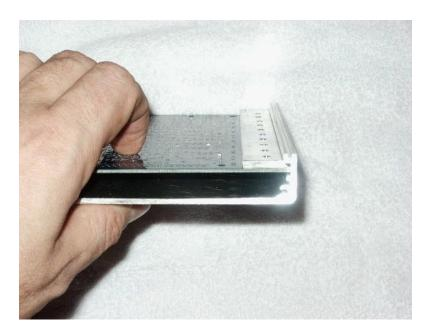
The wider lip of the case side is near the heat sink side of the board. This is to allow the top lid case to close. Mock it up by just sliding the board in the case with the end caps off, put on the top case half and slide the heat sink along the top, you will see why you need the fatter lip side of the bottom case half on the heat sink end. The aluminum should fit against the case lip for a little extra heat transfer.
