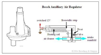
Mount the regulator to the engine such that engine heat can keep the valve closed when you do not need any additional air for warm up. During cold starts, the auxiliary air valve opens to allow additional air into the inlet duct. As engine heats up, a bi-metallic element expands and closes valve. At approximately 140°F (80°C) the auxiliary air orifice is completely closed by the valve.
