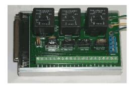
Whether you need the relay board depends on your ability and what you are comfortable with. MegaSquirt gets its power from the car's 12 Volt battery via pin 28 on the DB37 connector. The relay board, which is not required, makes it easier to hook up the wiring to MegaSquirt. It also reduces the chances that you will fry something in MegaSquirt through incorrect wiring.
