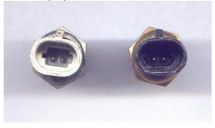
The wiring schematic for DB37 shows only one input for all of the sensors (except for the two for the TPS). The recommended GM sensors all have two wire connectors. The missing connection is a ground wire for the sensor. Sensor grounds should be brought to the same grounding point on the engine block as the MegaSquirt ground, unless they are grounded through the body of the sensor.
