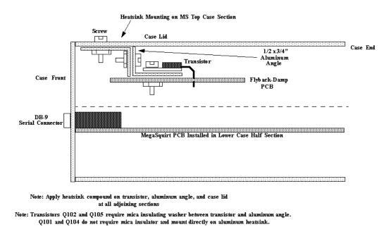
10) Bends the leads of the TIP125 Darlington transistors **Q102** and **Q105** so that the mounting holes and leads line up with both the PCB and heat-sink. **Make sure the leads of the transistor will not touch the heat sink!** The heat sink is sandwiched between the transistor body and the PCB.
