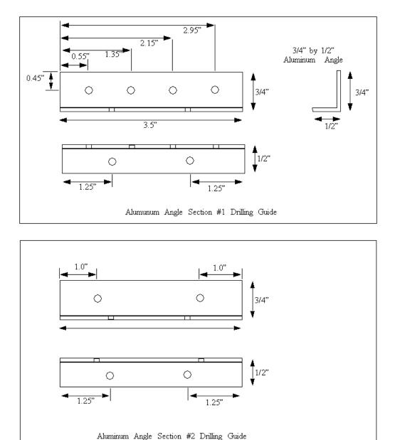
Make sure your heat sink is no longer than  $3\frac{1}{2}$ " (89mm), so that it can sit flat against the case. The edge of the heat sink is flush with the end of the case. Drill corresponding holes in the case. Be sure to drill the correct end of the case (the DB9/LED end). Verify that the heat sink will sit flat when bolted to the case.
