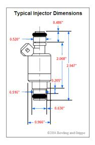
The manifold injector bungs are **0.530''-0.535''** inside diameter [about **17/32''** or **13.5 mm**]. The fuel supply rail bungs for the top of the injectors are the same size.
